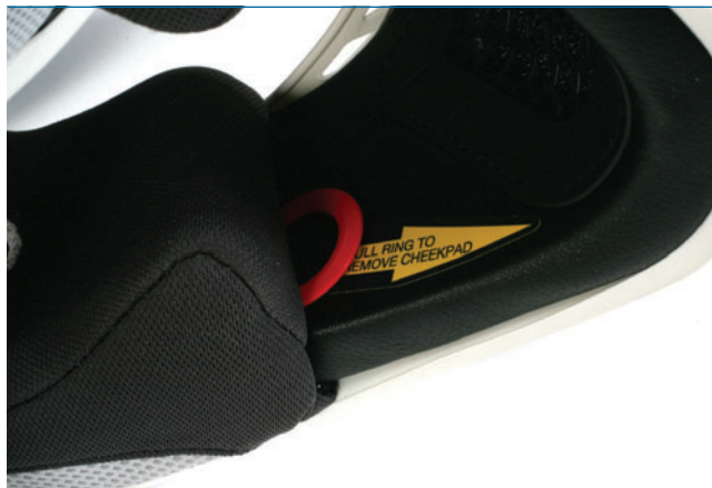
The cheek pad release is called the "Emergency Quick Release System." It allows a medical worker to pull the red rings and release the cheek pads, allowing the helmet to be removed with virtually no drag on the head, which reduces the trauma to the downed rider.
